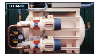
2 off CGG233R1/Y units on a 'domestic water module'. Duty approximately 2m<sup>3</sup>/h at 3 bar. This module distributes fresh water for domestic services such as toilets, showers, washbasins etc., on a tug currently based on the Solent. Built into the module is a calorifier for hot water service and U.V. treatment for potable (drinking) water.
