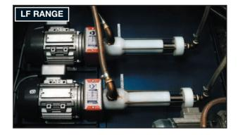
Various LF Range pumps playing an important role in furane binder systems, delivering a sulphuric or sulphonic acid (capacity up to 600 l/h and pressures up to 12 bar) to act as a catalyst on furane resin.
