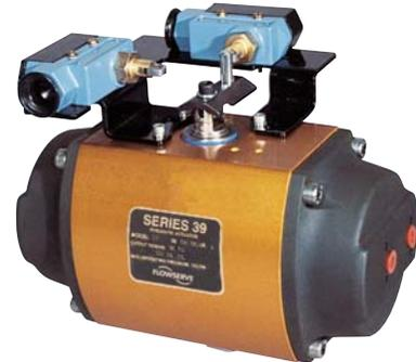
One or two switches can be furnished as required. The switch has a cast aluminum housing, SPDT switch, and a one-way roller lever. General Purpose (TYPE 1), Watertight (TYPE 1, 3, 3 R, and 4), and Hazardous Location (TYPE 7, Class I, Groups C and D; and TYPE 9, Class II, Groups E, F and G) housings are available.
