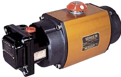
Where compact installation is required, an end-mounted limit switch module is available. This module comes as a combined Watertight TYPE 4 and Hazardous Location (Class I, Division 1, 2, Group C, D; and Class II, Division 1, 2, Group E, F, G) and comes with two SPDT or two DPDT mechanical switches. It is also available with SPST AC or DC proximity switches.
