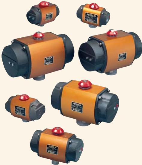
The Series 39 Pneumatic Actuator design is based on the opposed rack-and-pinion principle utilizing piston guide rods to guarantee part alignment. The fully supported guide rods minimize friction and wear between the pistons and the body bore.
