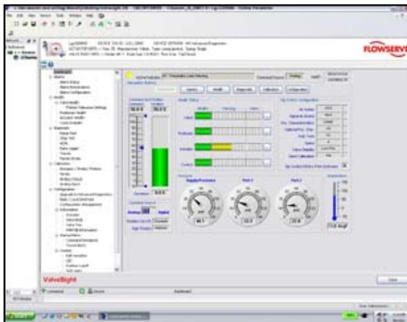
**The ValveSight Diagnostic Solution shows the “health” of your valve assembly on an easy to read Dashboard screen.**
