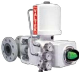
The VR is a piston actuator designed for supply pressures up to 150 psi (10.3 bar). It combines high torque and pneumatic stiffness for excellent throttling capabilities. This actuator is also field reversible.
