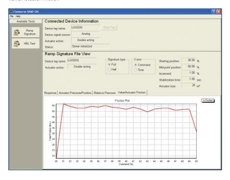
Plots the overall friction of the device. This is an excellent plot to use in determining the health of the valve.
