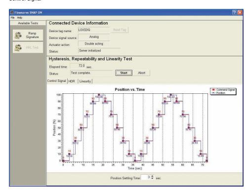
This measurement plots the device's Position vs. Command Signal. The X-axis is a user defined time increment between step changes. The Position Setting Time is set using the box directly below the graph.
