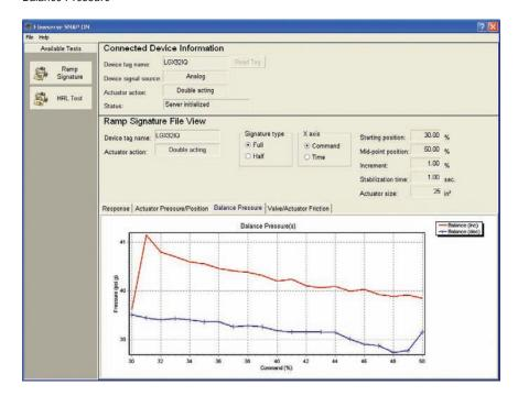
The balance pressure is (P1+P2)/2 for a double-acting actuator. Shifts in the balance pressure indicate an air leak in the actuator.
