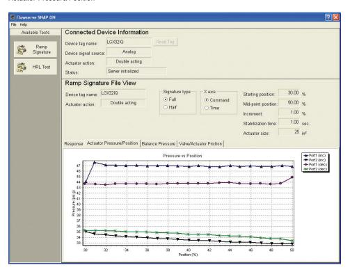
This plot isolates and expands the actuator pressures versus position for easier viewing.
