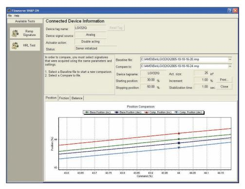
Three comparisons are made; Position, Friction, and Balance (balance pressure). When comparing signatures, Flowserve Snap-On will automatically verify that the signatures have the same starting and stopping point. If not, a comparison cannot be made between the two signatures. Easy-to-follow instructions on the screen will step the user through the process. First, select a baseline file, then select a second signature for comparison.
