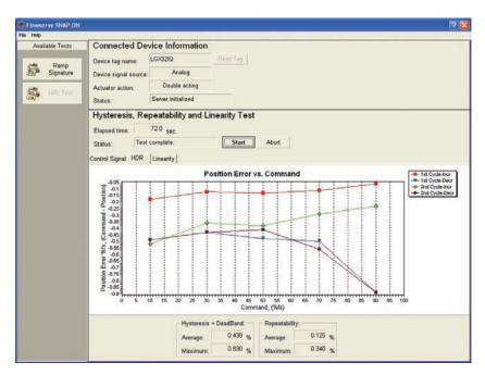
This measurement plots and calculates the hysteresis, deadband, and repeatability. The graph shows the Position Error vs. Command. The Y-axis is labeled "Position Error %" which is equal to the Command minus Position in percent. The X-axis is labeled Command as a percent of full stroke. Flowserve Snap-On then calculates the average and maximum combined hysteresis plus deadband and repeatability.
